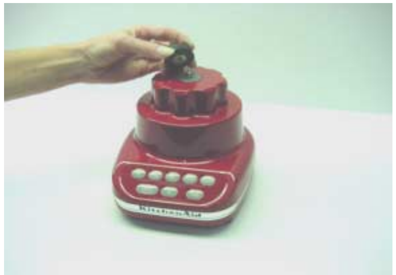
Fig.4 Install new coupler counter clockwise.
