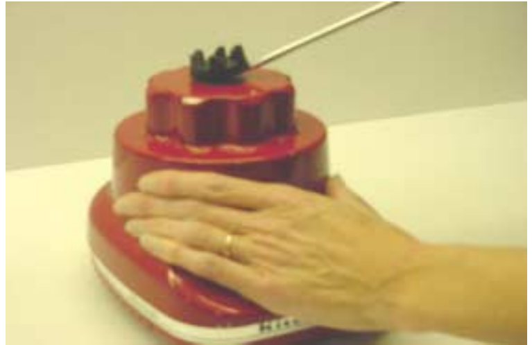
Fig. 2 Raise up on screw driver, bending coupler up.
