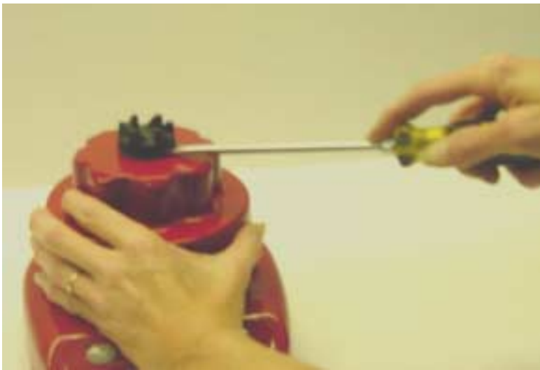
Fig. 1 Insert screw driver blade between coupler and blender housing; Approximately 1/2 inch.
